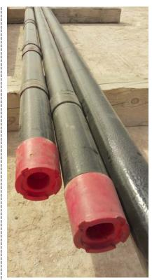
The Weatherford MetalSkin openhole liner can be used in the early stages of the well life cycle to preserve completion size in challenging drilling applications.
