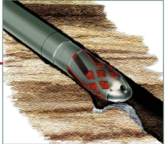
The *Diamondback* reamer shoe is designed to overcome obstructions and guide the casing to TD. Unlike a standard guide or float shoe, the *Diamondback* shoe is equipped with an eccentric profile nose which through rotation can climb ledges and negotiate obstructions. In addition, its cutting structure can open previously drilled wellbores that would otherwise be impassable due to sloughing or swelling formations.
