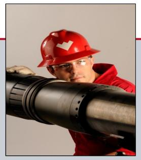
The Weatherford SwageSet liner-top packer provided a high-integrity seal between the annulus of the liner OD and the host casing ID, to prevent gas migration and flow while the cement set in an onshore well in Iraq. The successful installation of the Weatherford liner system products and services proved to be a reliable solution for a major oil and gas provider.
