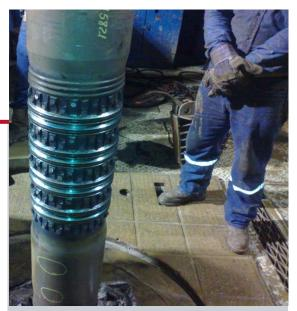
Weatherford's *TruForm* expandable liner hanger system, including the *DiamondBack* reamer shoe, were deployed to ream through a trouble zone, enabling EP Petrocecuador to successfully reach TD and isolate production sands.
