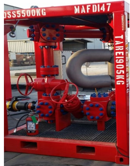
Managed pressure cementing—including the fully automated Victus Intelligent MPD System, Coriolis flowmeter, RCD 7875—successfully cemented the 7 5/8-in. liner.
