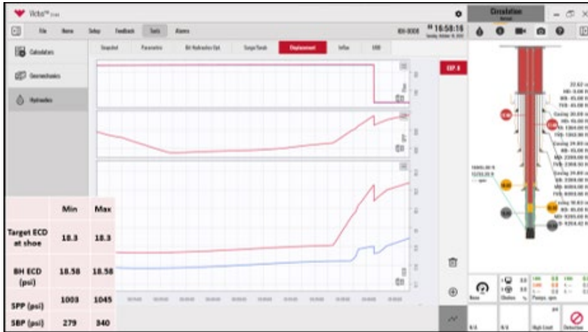
The pumping schedule of the managed pressure cementing of the 7 5/8-in. liner as displayed via a screenshot from the Victus simulation.
