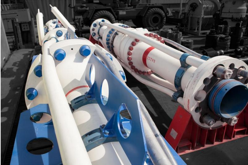
Weatherford prepared a deepwater MPD joint with auxiliary lines that enabled deployment below the tension ring and termination joint of the rig.
