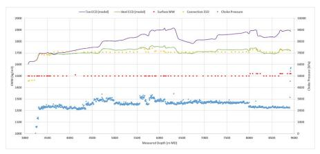
Engineering deliverables, monitored in real time, present important well construction parameters and provide accurate hydraulic plans.
