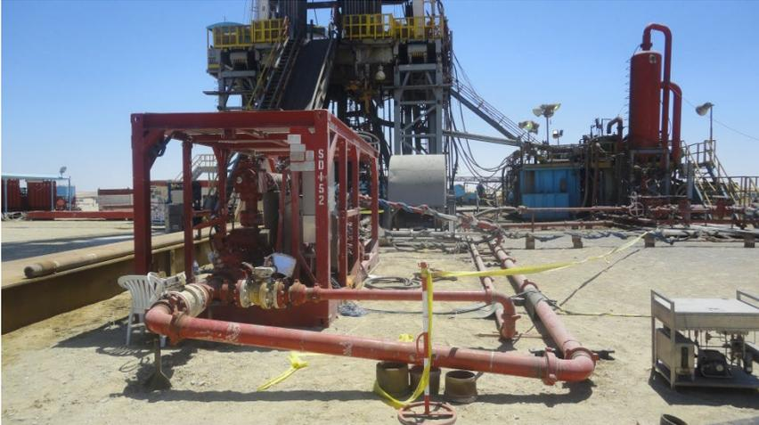
Used for the first time in an onshore well in Egypt, the Weatherford MPD control system enabled managed pressure drilling and managed pressure cementing operations.
