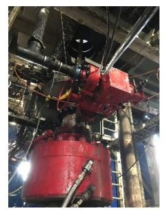
With the PressurePro system, the choke operator inputs the set point, and the choke automatically adjusts its position based on pressure or pump rate variations. Compared to manual or hydraulic systems that reactively apply surface backpressure, the choke provides more accurate and precise pressure control–within  $\pm 5$  psi ( $\pm 0.03$  MPa) of the pressure point set, and at a  $\pm 0.1\%$  fail-safe rate.
