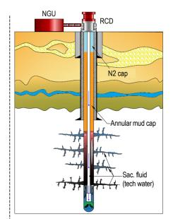
Weatherford introduced a nitrogen storage system with a nitrogen-generating unit on the location. The system connected to the well via the kill line to deliver instant nitrogen for nitrified PMCD operations.
