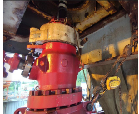
The critical component of any closed-loop drilling system—and the first line of defense for any wellbore—is the rotating control device (RCD). RCDs create a closed-loop environment to contain and divert fluids and to enable wellbore pressure management.
