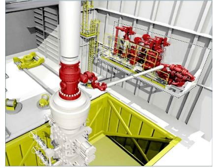
Mounting the new MPD installation against a wall near the moonpool facilitated direct access to the RCD for quick rig-up.
