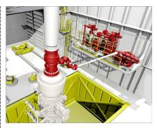
Mounting the new MPD installation against a wall near the moonpool facilitated direct access to the RCD for quick rig-up.
