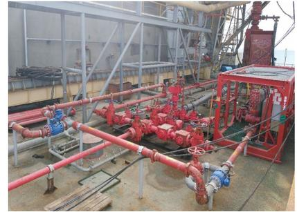
Managed pressure drilling equipment occupied only a small footprint on the platform.
