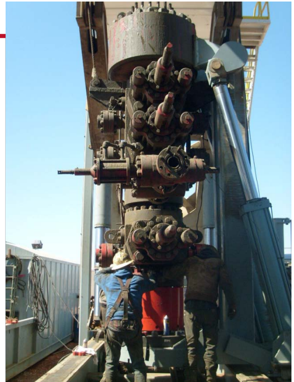
BOP stack and Rapid-Lock connector (red) mounted on the rig's BOP handler.
