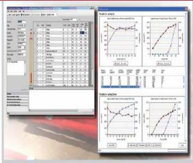
Weatherford uses stress-wave analysis to help examine or optimize the location of the jar in the drillstring or fishing assembly.
