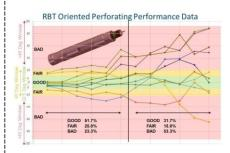
Comparison of perforation accuracy achieved with and without the relative bearing tool.
