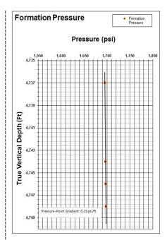
The figure shows the true vertical depth (ft) versus pressure levels (psi) in the well. The pressure-point gradient of 0.23 psi/ft indicates the presence of hydrocarbons.
