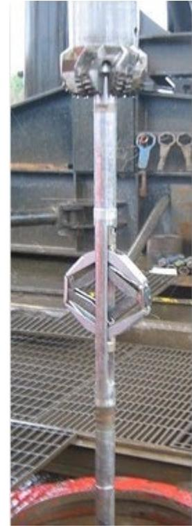
The Compact formation pressure tester (MFT) provided measurements to identify fluid contacts and determine permeability.
