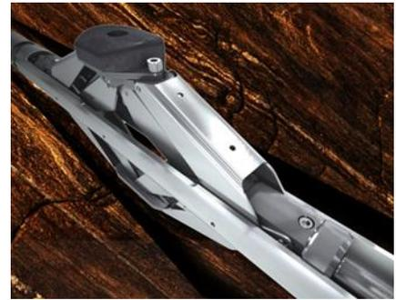
The slim, self-centering Compact formation pressure tester reduced the risk of sticking in a deviated hole with washouts.
