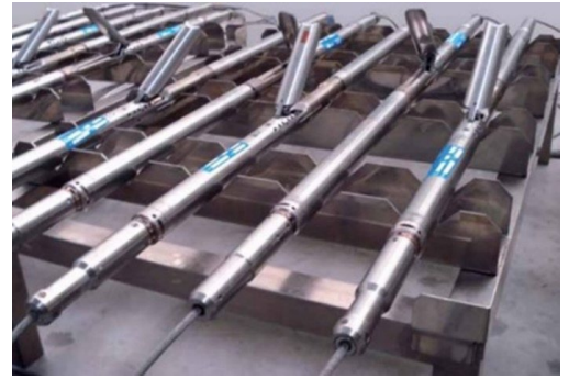
The Weatherford GAPS service is deployed in a cased borehole to profile the background noise levels throughout the length of the well. The background noise profile is analyzed to pinpoint areas with significant gas or water movement occurring behind the casing.
