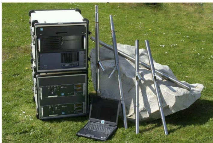
The Weatherford GAPS geophone array production survey tool is deployed in a cased borehole to profile the background noise levels throughout the length of the well. The background noise profile is analyzed to pinpoint areas with significant gas or water movement occurring behind the casing.
