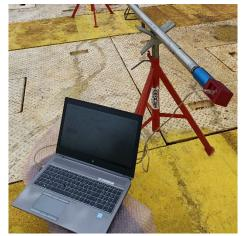
A single engineer, using a small, lightweight slickline deployment package, operates the Memory Raptor system, reducing operational complexity and enabling efficient, costeffective operations.
