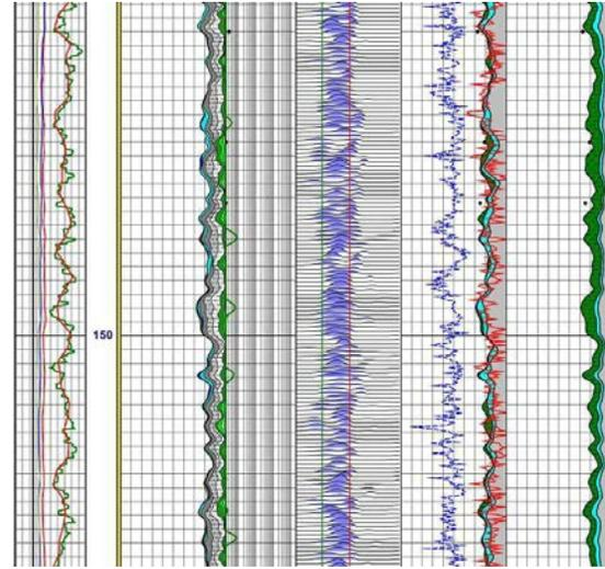
Above is a section of the Weatherford NMRT log, which helps determine clay-bound, capillary-bound, and free fluid (water) distributions. The log provided for log-to-core calibration after indicating a correlation with a core nuclear magnetic resonance (NMR) analysis. In the upper part of the hole, the NMR log showed a very high free-fluid content, which is a result of extreme washout.
