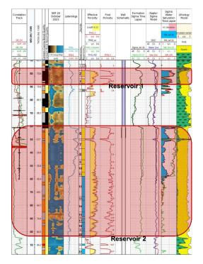
The log plot of complex openhole petrophysical analysis and the time-lapsed cased-hole logs (captured by the Raptor 2.0 system) for monitoring the fluid contacts.
