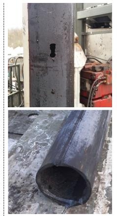
The wireline solution enhanced operational safety by avoiding the use of hazardous chemicals or explosives. The top image shows the perforation, and the bottom image shows the cut, made with non-explosive tools.
