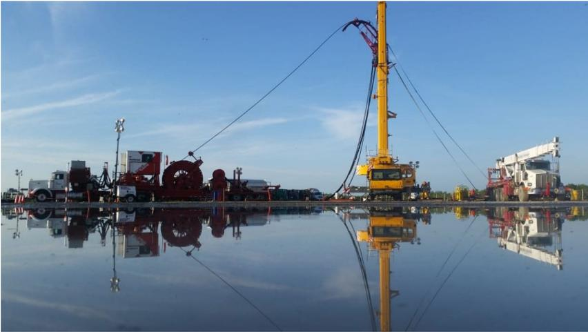
The above photo shows the coiled-tubing unit used to run formation evaluation tools, perform sand jetting, and mill multiple frac plugs in between 17 stages of hydraulic fracturing treatments.
