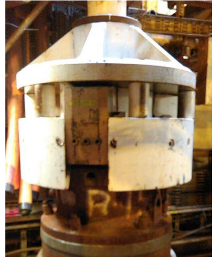
The image shows the M.O.S.T. Plus system, a proven subsea wellhead recovery tool that latches onto the external profile of a subsea wellhead while a hydraulic internal casing cutter cuts the conductors.
