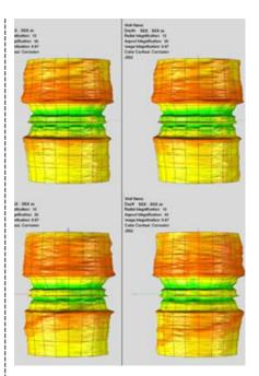
URS data is presented in 3D format for interactive evaluation and easy visualization. The above imaging shows that the inside and outside of the casing are intact with no evidence of corrosion or pitting.
