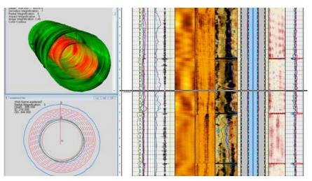
For precise interpretation of CIT data, each collar and hardware is imaged every 90° around the casing. In the resulting images above, the collars show no anomalies.
