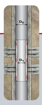
Weatherford provided an operator two customdesigned *MetalSkin* cased-hole liner systems incorporating high-temperature, swellable hybrid elastomers to isolate existing perforations in two separate oil and gas producing wells in California.
