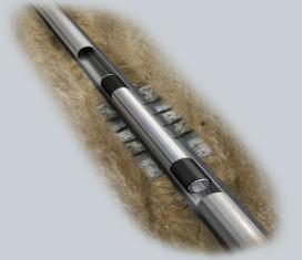
The second installation of Weatherford's *MetalSkin* system in Malaysia provided permanent isolation to a damaged casing interval, enabling the well to be recompleted as a water-alternating-gas injector.
