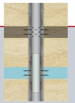
The Weatherford MetalSkin cased-hole liner system provided the solid-expandable solution with permanent isolation and a larger ID for improved production.
