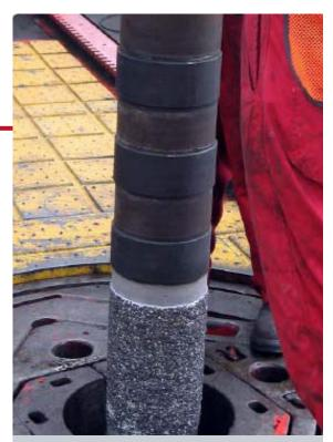
Weatherford's *MetalSkin* cased-hole liner system provides a permanent, cost-effective solution, isolating and sealing unwanted perforations for increased production capacity.
