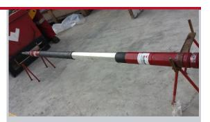
The Weatherford E-IRBP was deployed via coiled tubing to shut off a water-producing zone in an onshore gas well. This intervention enabled more than US \$2 million in production.
