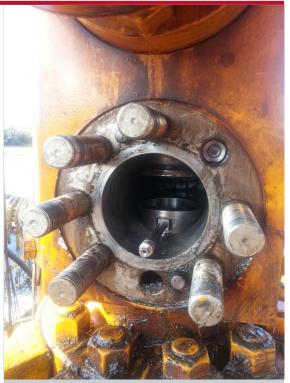
Weatherford's *REN-Gate* is a new wellhead penetration that enters through the lower master valve (LMV) bonnet and lower seat, providing the communication port to the control line hanger and capillary tubing to function the *Optimax* safety valve. The picture above shows the new LMV lower seat and capillary tube mid-installation.
