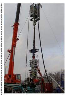
The Renaissance WDCL system replaced a leaking SCSSV in three wells without using a rig or requiring major workovers. The operation restored oil production to original rates in the three wells and saved US \$20 million.
