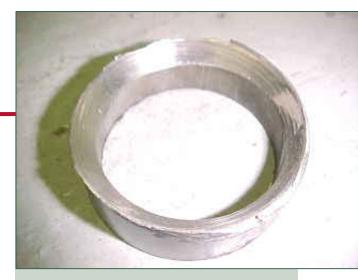
Weatherford's hydraulic tubing cutter quickly restored production, cutting this ultra-hard tail pipe section (above) in less than 15 min. This tool is designed to mechanically cut tubing, drillpipe, or other tubulars. The cutter is flow actuated and mechanically rotated by a motor or through surface methods. It can be used in all coiled-tubing applications to assist stabilization and centralization of the BHA for a cleaner, quicker cut.
