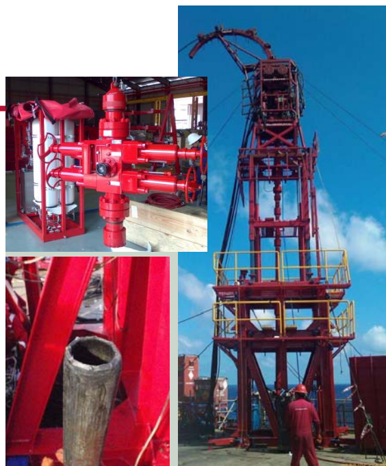
Pictured clockwise from top left: Weatherford's dual-barrier deployment system, coiled tubing rig-up with deployment system, 1 1/2-in. coiled tubing after being snipped by cutting overshot.
