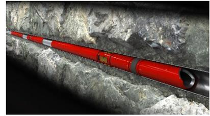
The Weatherford WidePak straddle system is a high-pressure packer used for temporary or permanent isolation of tubing sections, perforations, or windows. Its large packer throughbore is set in one run using slickline and enables maximum production after setting as well as many intervention operations.
