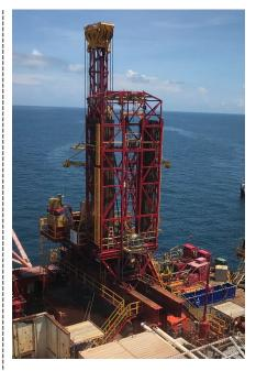
The Weatherford Rig-Free pulling-and-jacking unit provides a foundation for offshore well abandonment and intervention operations.
