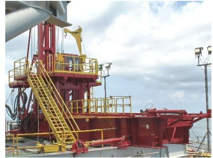
Weatherford's pulling-and-jacking unit situated on the wedge deck during decommissioning operations at the well site in the Gulf of Mexico.
