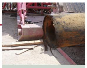
Designed to cut tubing of various grades and internal diameters, the Weatherford hydraulic tubing cutter can also be dressed with inserts to cut drillpipe, as was done on this job.
