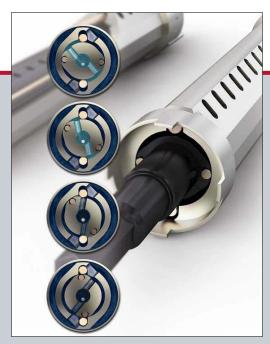
Weatherford's *MacDrill* motor is a revolutionary high-temperature hydraulic motor for milling and well-cleaning operations. The motor works on the positive-displacement principle but features a stainless-steel stator rather than the elastomers found in conventional motors. With no elastomer in the stator, the motor can operate at temperatures up to 500 F (260 C) and can be powered by hydrocarbon-based solvents, acids, and gases.
