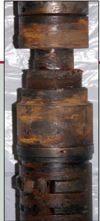
Weatherford 2 1/8-in. thru-tubing bottomhole assembly with impact hammer, retrieving spear, and 3-in. Camco lock mandrel (no fishing neck ).
