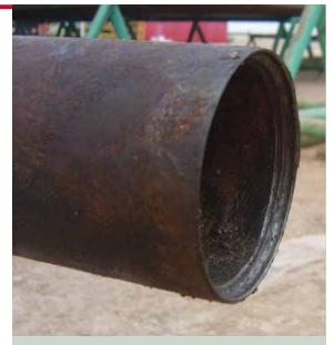
The tubing cutter performed a very clean cut, regardless of thickness and deviation.
