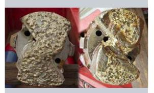
Weatherford milled 109 ft (33.2 m) of a cemented 3 1/2-in. tubular at a ROP of 8 ft/hr (2.4 m/hr), enabling the operator to sidetrack the well and regain production from a strategic reservoir and eliminating the need to drill a second well. The two-pod mill dressed with *CustomCut* inserts performed well with nominal wear. The left photo shows the first two-pod mill before it was deployed, and the right photo shows the two-pod mill after it milled 94 ft (28.6 m).
