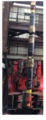
The image at the left shows a unique bottomhole assembly designed to remediate annuli with OBM in a cost-effective manner while preserving the offshore location.
