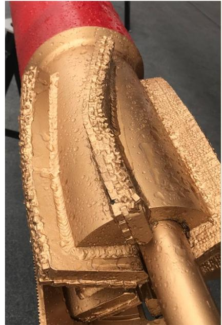
The Weatherford AlphaST system uses a lead mill (shown above) and a flex mill to make a quick departure from the original wellbore.
