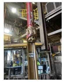
The AlphaV milling assembly ready to be run on rigfloor in the North Sea. This casing exit system eliminates wellbore preparation runs by including a gauge mill and scraper assembly on the toolstring. AlphaV increases tripping speeds by replacing traditional shear bolts with the patented HMR system to enable high-torque and load-bearing capabilities.
