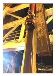
The AlphaV casing-exit system eliminates wellbore preparation runs by including a gauge mill and scraper assembly on the toolstring. The system increases tripping speeds by replacing traditional shear bolts with the HMR system to enable high-torque and loadbearing capabilities.
